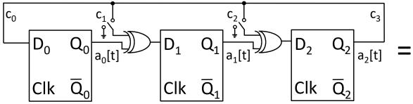
Example 3: Consider an LFSR (with the notation as defined) with n=3,  $c_2=0$  and  $c_1=0$ .
