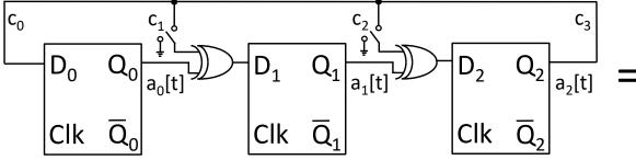
Example 2: Consider an LFSR (with the notation as defined) with n=3,  $c_2=1$  and  $c_1=0$ .
