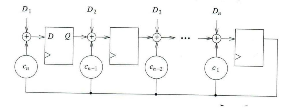
Figure 10.17 Multiple-input signature register
