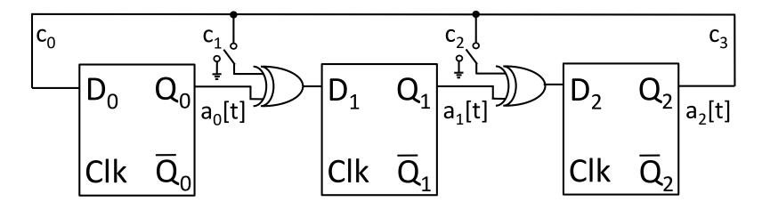
$A(x)[t] = \langle a_{n-1}[t], \dots, a_2[t], a_1[t], a_0[t] \rangle$  which can be represented in polynomial space as  $\sum_{i=0}^{n-1} a_i x^i = a_{n-1} x^{n-1} + \dots + a_2 x^2 + a_1 x + a_0$
