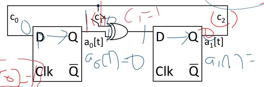
•  $f(x)[t] = a_1[t]x + a_0[t]$ ,  $P(x) = c_2x^2 + c_1x + c_0$   $f(x)[t+1] = xf(x)[t] \mod P(x)$ ©Georgia Institute of Technology, 2018-2025
