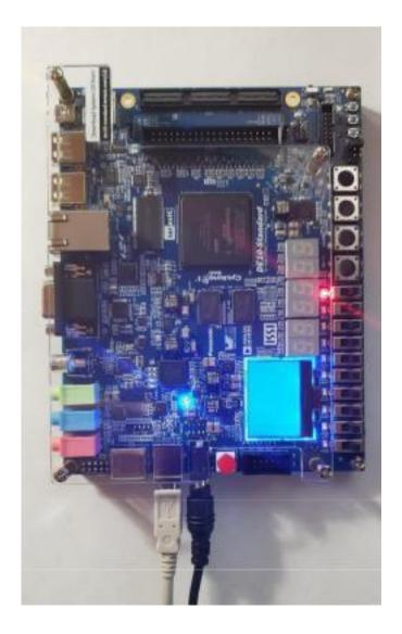
The term "Programming" is used by Quartus, and we will use it as well to minimize confusion. But you should always think of this as "configuring" the FPGA to connect its logic, flip-flops, and other hardware internally. There is no program "running" on the board -- it will be implementing hardware.
