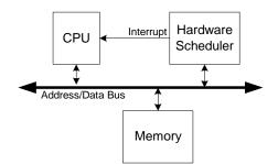
Figure 6. The hardware scheduler connected as an I/O device.
