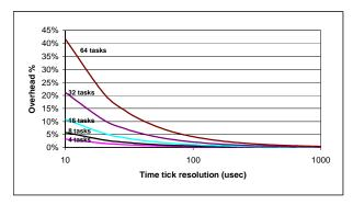
Figure 8. The scheduler and the time tick processing overheads in MicroC/OS II.
