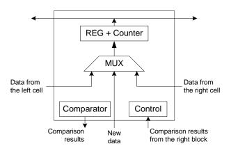
Figure 3. The PQ cell architecture.
