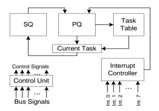
Figure 1. The configurable hardware scheduler micro-architecture.
