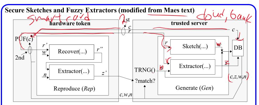
This PUF-based authentication protocol shows the *hardware token*, e.g., smart card, shown on the left and the *secure server*, e.g., bank, shown on the right
