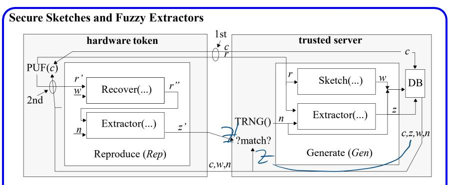
The output r" of Recover and the seed n are used by the Extractor to generate z'
