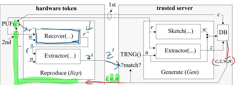
Authentication in the field begins by selecting a tuple (c, z, w, n) from the DB and transmitting the challenge c, helper data w and the seed n to the hardware token
