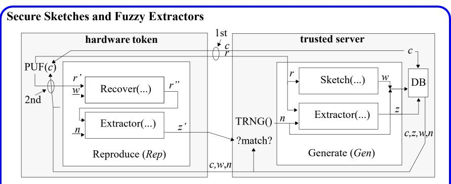
Authentication in the field begins by selecting a tuple (c, z, w, n) from the DB and transmitting the challenge c, helper data w and the seed n to the hardware token
