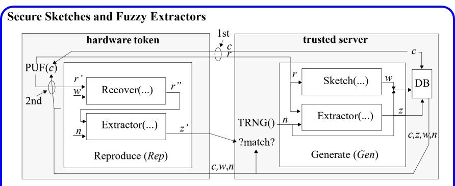
The *Extractor* takes both *r* and a random number (seed) *n* and produces an *entropy distilled* version *z*
