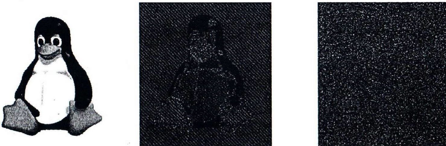
FIGURE 3.6: An illustration of the dangers of using ECB mode. The middle figure is an encryption of the image on the left using ECB mode; the figure on the right is an encryption of the same image using a secure mode. (Taken from http://en.wikipedia.org and derived from images created by Larry Ewing ( lewing@isc.tamu.edu ) using The GIMP.)
